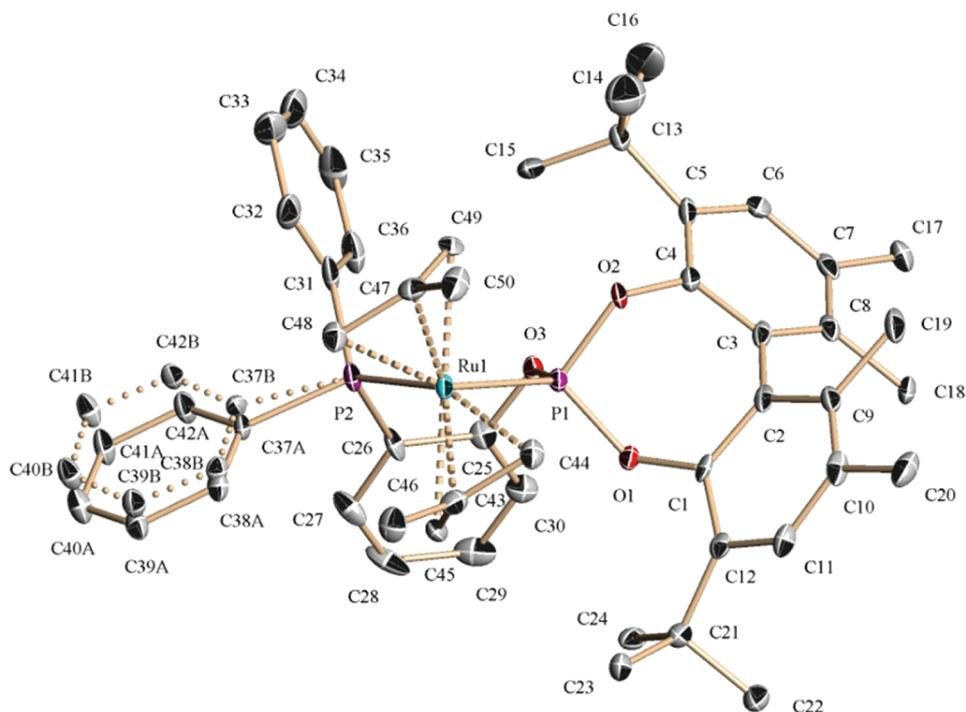
**Figure 2.** ORTEP view of complex **1a**. Selected bond lengths (Å) and angles (deg): Ru(1)–C(47) = 2.179(3), Ru(1)–C(48) = 2.261(3), Ru(1)–C(49) = 2.213(4), Ru(1)–P(1) = 2.2227(11), Ru(1)–P(2) = 2.3095(10); P(1)–Ru(1)–P(2) = 89.45(4), C(49)–Ru(1)–P(1) = 90.67(10), C(45)–Ru(1)–P(1) = 93.50(9), P(1)–Ru(1)–C(44) = 87.13(10), C(45)–Ru(1)–P(2) = 89.79(10), C(48)–Ru(1)–P(2) = 88.55(10).
