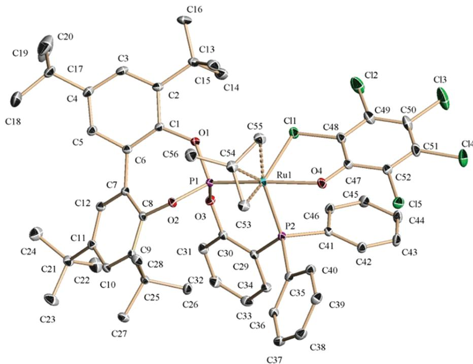
**Figure 7.** ORTEP view of complex **3h**. Selected bond lengths (Å) and angles (deg): Ru(1)–C(53) = 2.134(2), Ru(1)–C(54) = 2.254(2), Ru(1)–C(55) = 2.302(2), Ru(1)–O(4) = 2.1731(15), Ru(1)–Cl(1) = 2.4924(6), Ru(1)–P(1) = 2.1607(5), Ru(1)–P(2) = 2.3061(6); C(53)–Ru(1)–P(1) = 98.75(7), C(53)–Ru(1)–O(4) = 90.53(8), P(1)–Ru(1)–O(4) = 168.69(5), P(1)–Ru(1)–C(55) = 109.95(7), C(53)–Ru(1)–P(2) = 99.28(7), P(1)–Ru(1)–P(2) = 89.91(2).
