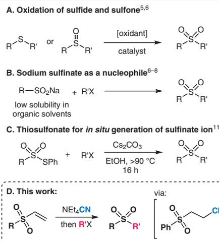
**Scheme 1** Conventional routes to access sulfones: (A) Oxidation of sulfides and sulfoxides, (B) nucleophilic substitution reaction of metal sulfonates, and (C) thiosulfonates to generate sulfonates. (D) This work represents devinylation to access nucleophilic sulfinate ions for substitution reactions.
