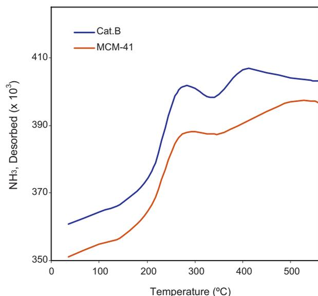
**Fig. 4.** Temperature programmed desorption analysis (TPD) of the absorption  $\text{NH}_3$  of Cat. B and MCM-41.
