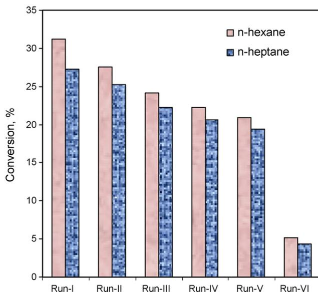
**Fig. 8.** Recycle testes of Cat. **B** in the course of *n*-alkanes hydroisomerization (conditions as in Table 1).
