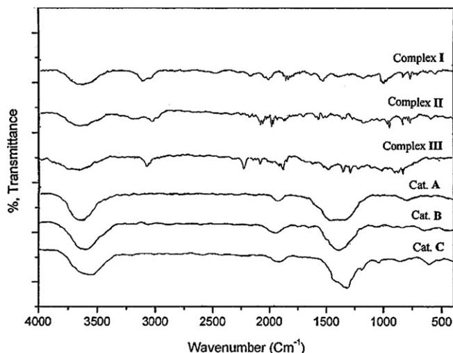
Fig. 1. FT-IR of Re complexes I–III and after immobilized on modified MCM-41 as Catal. A to Catal. C.
