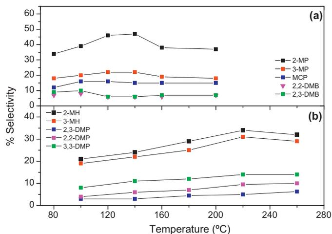
**Fig. 5.** Temperature effect on the percentage selectivity of the isomerized products of *n*-hexane (a) and *n*-heptane (b), in the presence of the Cat. **B** (constant conditions: catalyst; 25 mg,  $p(\text{H}_2)$ ; 2 atm, *n*-alkane; 3.0 mL; 12 h for *n*-hexane and 18 h for *n*-heptane).
