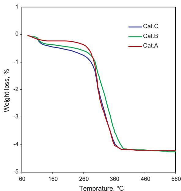
Fig. 3. TGA analysis results of single site immobilization of Re complexes over MCM-41 Cat. **A** to **C**.
