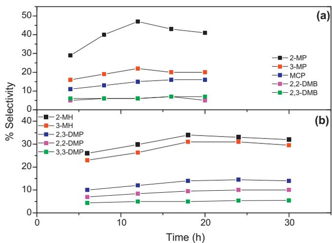
**Fig. 6.** Time effect on the percentage selectivity of the isomerized products of *n*-hexane (a) and *n*-heptane (b), in the presence of the Cat. **B** catalyst (constant conditions: catalyst; 25 mg,  $p(\text{H}_2)$ ; 2 atm, *n*-alkane; 3.0 mL; at 140 °C for *n*-hexane and at 220 °C for *n*-heptane).
