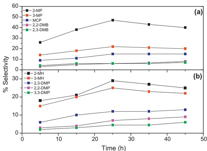
**Fig. 7.** Cat. **B** amount effect on percentage selectivity of the isomerized products of *n*-hexane (a) and *n*-heptane (b) (constant conditions:  $p(\text{H}_2)$ ; 2 atm, *n*-alkane; 3.0 mL; 12 h for *n*-hexane at 140 °C and 18 h for *n*-heptane at 220 °C).
