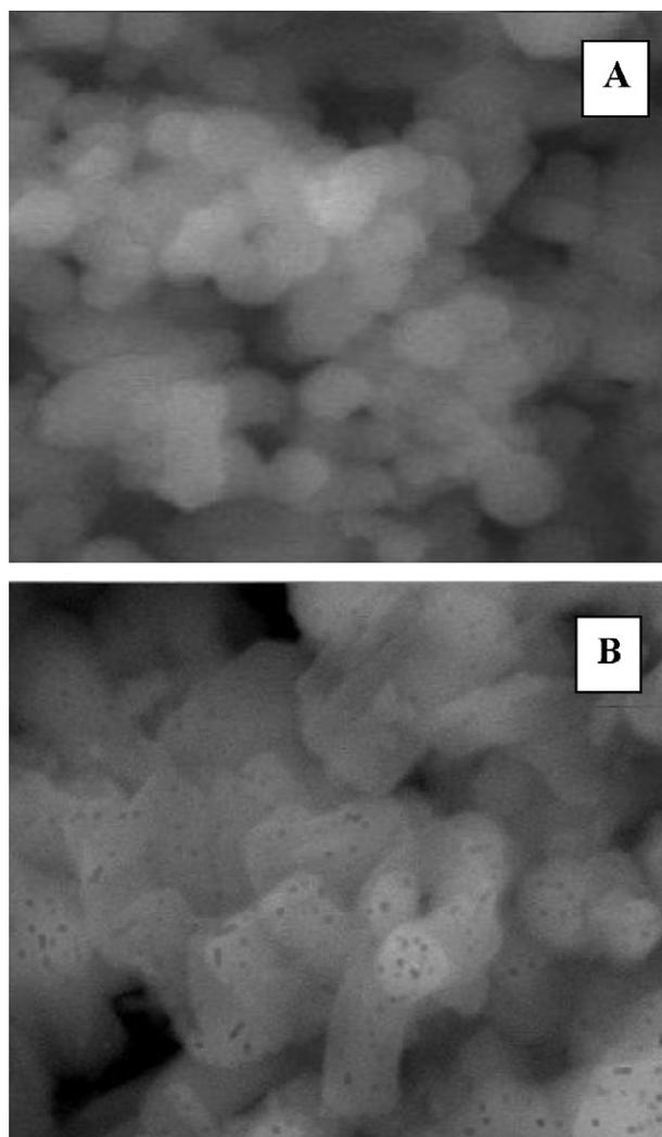
Fig. 2. Scanning electron microscopy morphological study (20,000× magnification) of (a) modified MCM-41 and (b) MCM-41 immobilized Cat. **B**.
