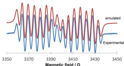
**Figure 3.** Experimental (gray) and simulated (black) X-band EPR spectra of **3** in toluene/THF solution at room temperature. G = gauss.
