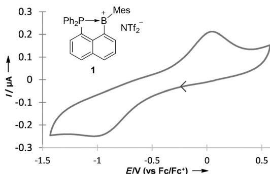
**Figure 2.** Cyclic voltammogram of **1** in a fluorobenzene solution containing  $[\eta\text{Bu}_4\text{N}][\text{NTf}_2]$  (0.06 M) as the electrolyte. Scan rate: 500 mV s $^{-1}$ ; potential reported against  $\text{Fc}/\text{Fc}^+$  as the internal standard.
