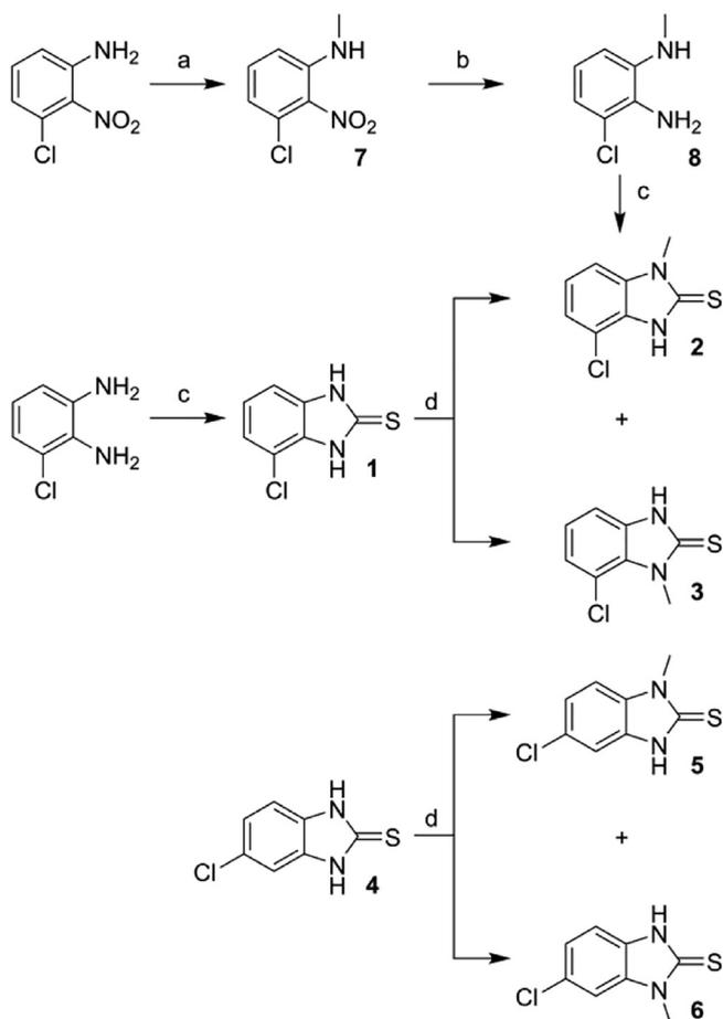
**Scheme 1.** Synthesis of chlorinated benzimidazole-2-thione derivatives. Reagents and conditions: (a) MeI, NaH, DMF, 0 °C, 1 h, 47% yield; (b) Fe, HCl (37%), EtOH, 80 °C, 6 h, 76% yield; (c) potassium ethyl xanthate, EtOH (96%), H<sub>2</sub>O, 80 °C, overnight, 27% yield for **1**, 16% yield for **2**; (d) i) TrCl, TEA, anhydrous THF, Ar, rt, overnight; ii) MeI, KOH, acetone, rt, 2–5 h; iii) 5% AcOH in MeOH, 65 °C, 30 min, 58% yield for **2** and **3**, 73% yield for **5** and **6**.
