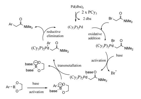
Scheme 1. Plausible mechanism of the Suzuki-type reaction to form  $\alpha$ -arylamide.
