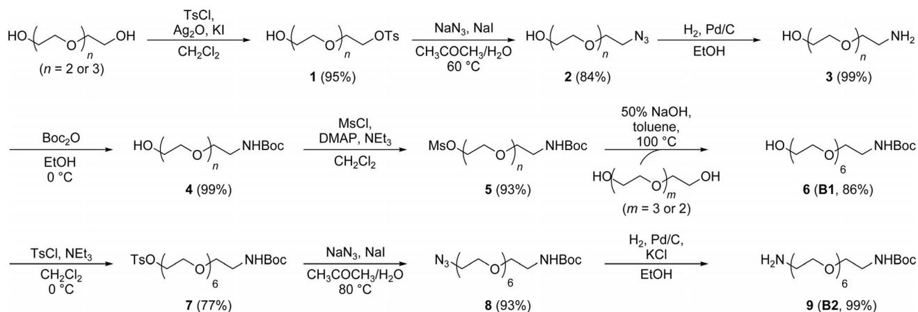
Scheme 1. Synthesis of  $\alpha,\omega$ -functionalized EG heptamers. TsCl = tosyl chloride; Boc = *tert*-butyloxycarbonyl; MsCl = mesyl chloride; DMAP = dimethylaminopyridine.
