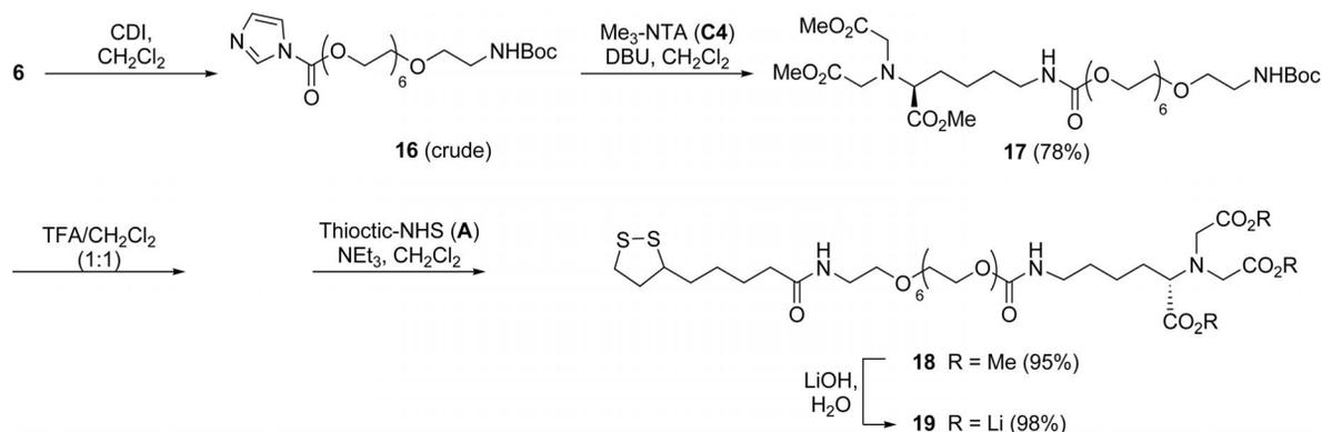
Scheme 3. Synthesis of linker assembled with **6**. CDI = carbonyldiimidazole; DBU = diazabicycloundecane.
