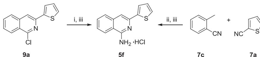
**Scheme 2.** Synthesis of 3-heteroarylisquinolinamine **5f**. Reagents and conditions: (i) NH<sub>4</sub>OH, NaHCO<sub>3</sub>, DMF,  $50\text{ }^{\circ}\text{C}$ ; (ii) LiNMe<sub>2</sub>, HMPA, dry THF,  $-78\text{ }^{\circ}\text{C}$ ; (iii) *c*-HCl, acetone.
