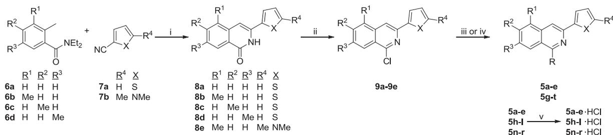
**Scheme 1.** Synthesis of 3-heteroarylisquinolinamines **5**. Reagents and conditions: (i) *n*-BuLi, dry THF,  $-78\text{ }^{\circ}\text{C}$ ; (ii) POCl<sub>3</sub>,  $50\text{ }^{\circ}\text{C}$ ; (iii) Amine, K<sub>2</sub>CO<sub>3</sub>, DMF,  $110\text{ }^{\circ}\text{C}$ ; (iv) NaN<sub>3</sub>, DMF,  $100\text{ }^{\circ}\text{C}$ ; (v) *c*-HCl, acetone.
