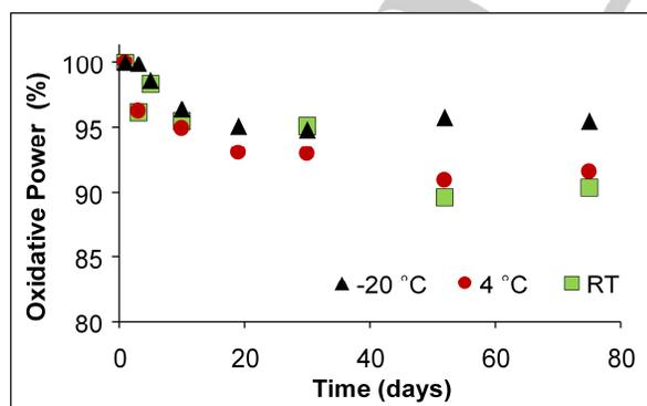
**Figure 9.** Oxidative power of polycrystalline  $\text{Cy}_3\text{PO}-(\text{HOO})_2\text{CMeEt}$  (**4**) after being stored at the indicated temperatures. 100% oxidative power is equivalent to 2 moles of active oxygen per mole of **4**.
