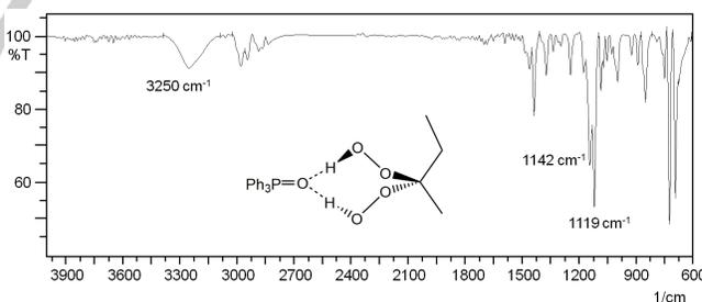
**Figure 2.** IR spectrum of polycrystalline  $\text{Ph}_3\text{PO} \cdot (\text{HOO})_2\text{CMeEt}$  (**3**).
