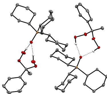
**Figure 6.** Single crystal X-ray structure of C<sub>3</sub>PO·(HOO)<sub>2</sub>CMePh (**7**, two independent molecules).<sup>[34]</sup> Thermal ellipsoids are shown at the 50% probability level. Only the hydrogen-bonded H atoms are shown for clarity.
