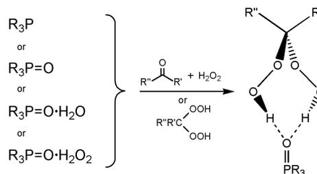
**Scheme 3.** General synthesis routes for di(hydroperoxy)alkane adducts of phosphine oxides.
