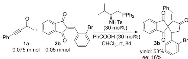
Scheme 2. Reaction catalyzed by L-valine-derived phosphine.
