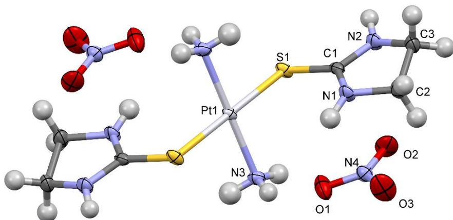
**Figure 1** A view of the molecular structure of **1** with atomic labelling. The displacement ellipsoids are drawn at the 50% probability level. Atoms not labelled are related by inversion symmetry
