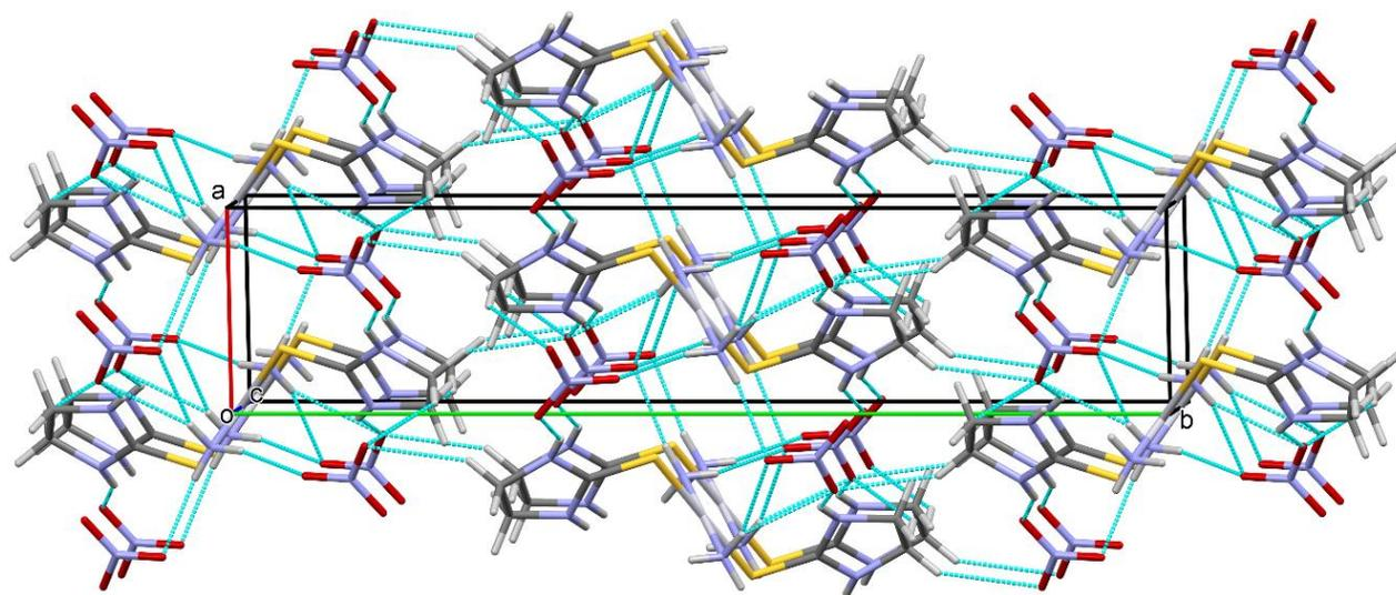
**Figure 3** The crystal packing of **1**, viewed along the *c* axis. The N–H...O, N–H...N and C–H...O hydrogen bonds are shown as dashed lines and lead to the formation of a three-dimensional structure.
