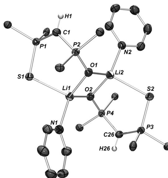
Figure 1. ORTEP plot of compound **6**<sub>Li</sub>; ellipsoids are set at 50% probability. Hydrogen atoms (except for H1 and H26) and the phenyl rings (except for the *ipso* carbon atoms) on the P atoms have been omitted for clarity. Selected bond lengths [Å]: C1–P1 1.721(3), C1–P2 1.703(3), P1–S1 1.994(1), P2–O1 1.524(2), O1–Li1 1.951(5), O1–Li2 1.922(5), C26–P3 1.721(3), C26–P4 1.702(3), P3–S2 1.992(1), P4–O2 1.523(2), O2–Li1 1.910(5), O2–Li2 1.922(5).
