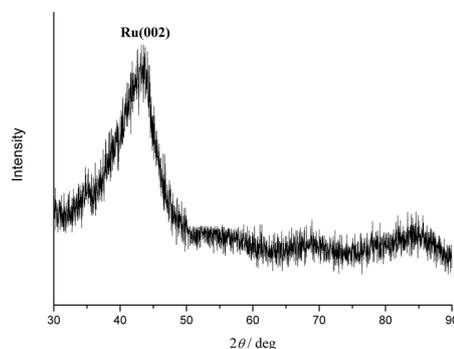
Fig. 3 X-Ray diffraction pattern of isolated Ru NPs 1.
