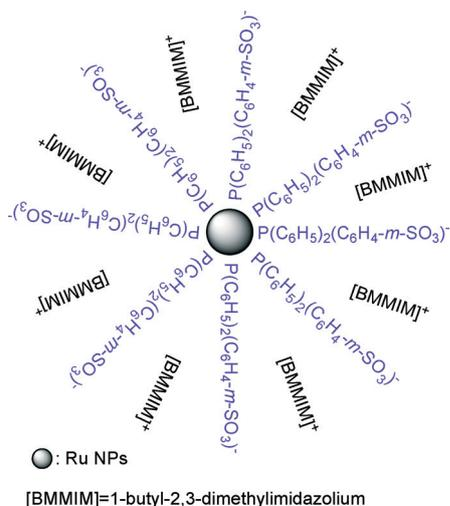
Fig. 4 The PFIL ([BMIM][tppm]) stabilized/modified Ru nanoparticles.
