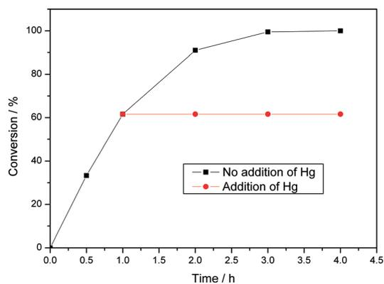
Fig. 5 Reaction profiles for hydrogenation of styrene and Hg<sup>0</sup> poisoning of Ru NPs 1. Reaction conditions: styrene ( $8.9 \times 10^{-3}$  mol; styrene/Ru = 500), 30 °C, H<sub>2</sub> at 1 MPa.
