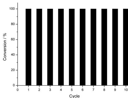
Fig. 6 Recyclability of Ru NPs 1 for the hydrogenation of styrene. Reaction conditions: styrene ( $8.9 \times 10^{-3}$  mol; styrene/Ru = 500), 30 °C, H<sub>2</sub> at 1 MPa.
