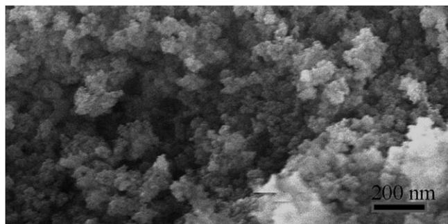
**FIGURE 8** SEM image of recovered catalyst after reaction
