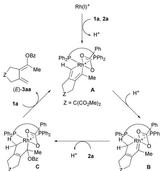
**Scheme 1** Possible mechanism for the formation of **3aa**.
