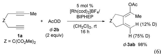
In conclusion, we have demonstrated cationic rhodium(I)/bisphosphine complex-catalyzed chemo-, regio-, and stereoselective cyclizations of 1,6-diyne with carboxylic acids, leading to cyclic diene carboxylates. Importantly, the present rhodium-catalyzed diyne cyclization allows the use of both terminal and internal diynes, proceeds under mild reaction conditions, and is specific to carboxylic acids.
