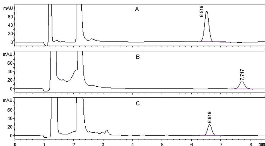
Fig. 4. HPLC chromatograms of (*R*)-MTPA esters of dimethyl malates, eluted with an isocratic methanol/water system (65:35, v/v) at 1 mL/min and monitored at 220 nm. A, B and C present the products prepared from standard *D*-malic acid, standard *L*-malic acid, and the hydrolyzate of **1**, respectively.
