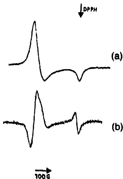
Fig. 2. X-band ESR spectra recorded on a CH 2 Cl 2 sample solution of 2b withdrawn at the first stages of controlled potential electrolysis (0.3 electron/molecule at E_a = +0.5 \text{ V} ) performed at 253 K. (a) First derivative spectrum recorded at liquid nitrogen temperature (100 K); (b) second derivative mode.
