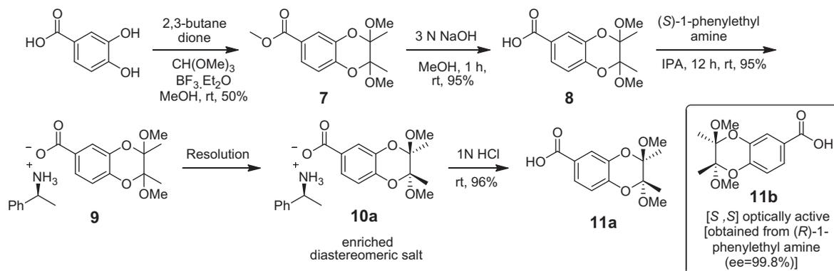
Scheme 2. Synthesis of chiral benzoic acids.
