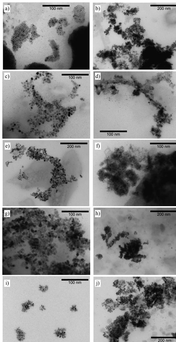
**Figure 1.** TEM images of PEG/Pd nanoparticles obtained after Mizoroki-Heck reaction (left column) and without substrates (right column) in different PEG: a-b) PEG-1100-OH; c-d) PEG-2000-OH; e-f) PEG-3400-OH; g-h) MeO-PEG-2000-OH; i-j) MeO-PEG-2000-OMe.
