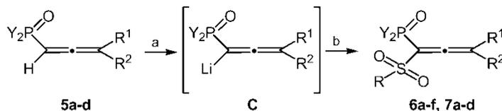
**Scheme 3.** Synthesis of 1-sulfonyl-substituted phosphorylated allenenes. Reagents and conditions: a) LDA, THF,  $-78^\circ\text{C}$ , 1 h; b)  $\text{RSO}_2\text{Cl}$  (R = Me,  $\text{CCl}_3$ , TMSO), THF,  $-78^\circ\text{C}$  to rt, 1 h.
