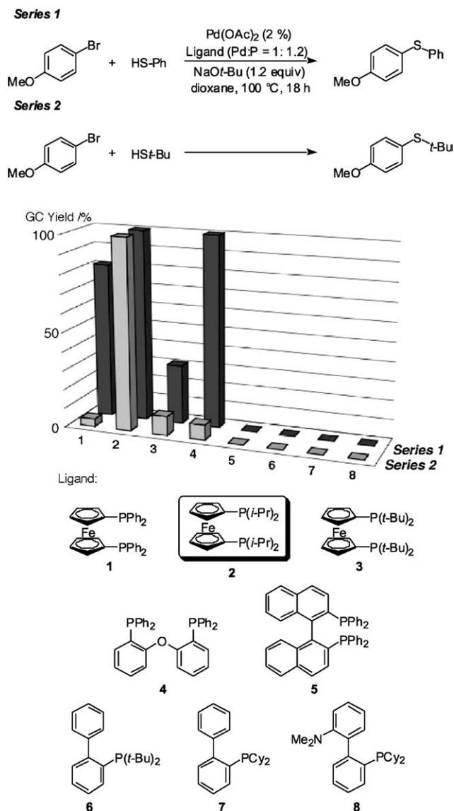
**Figure 1.** Screen for ligand efficiency in Pd-catalyzed C–S bond-forming reactions. Reaction conditions: ArBr (1.0 mmol), RSH (1.0 mmol), Pd(OAc)<sub>2</sub> (2.0 mol%), Ligand (Pd/P=1.0/1.2), *t*-BuONa (1.2 mmol) in dioxane (2 mL) at 60 °C for 18 h.
