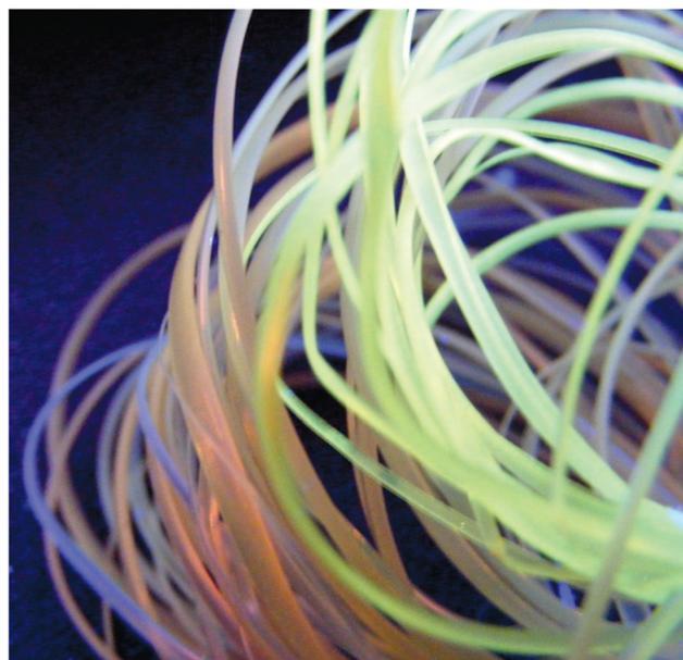
**Fig. 2** Extruded phosphorescent polypropylene doped with complex 2c (green) and 2a (orange).
