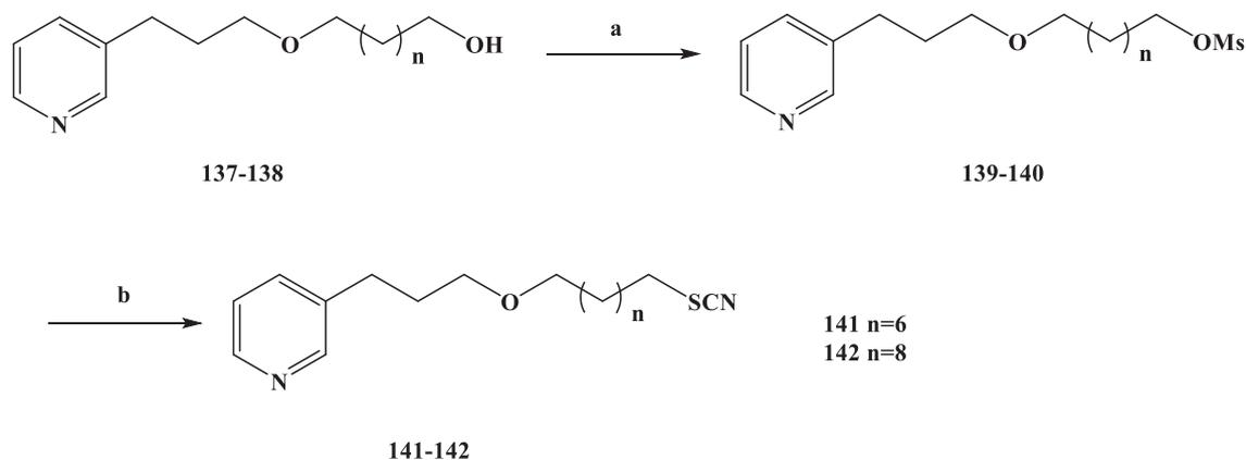
**Scheme 6.** Synthesis of compounds **141** and **142**. Reagent and conditions: (a) MsCl, Et<sub>3</sub>N, CH<sub>2</sub>Cl<sub>2</sub>, r.t., 10 h; (b) TBAB, KSCN, THF, reflux, 3 h.
