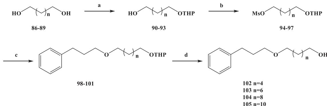
**Scheme 3.** Synthesis of 3-alkylpyridine marine alkaloid analogues compounds **102–105**. Reagent and conditions: (a) NaHSO<sub>4</sub>, DHP, DMSO, hexane, 40 °C, 16 h; (b) MsCl, Et<sub>3</sub>N, CH<sub>2</sub>Cl<sub>2</sub>, r.t., 10 h; (c) 3-(pyrid-3-yl) propan-1-ol, NaOH/H<sub>2</sub>O, Bu<sub>4</sub>N<sup>+</sup>Br<sup>-</sup>, Et<sub>2</sub>O, r.t., 72 h; (d) MeOH, HCl, r.t., 12 h.
