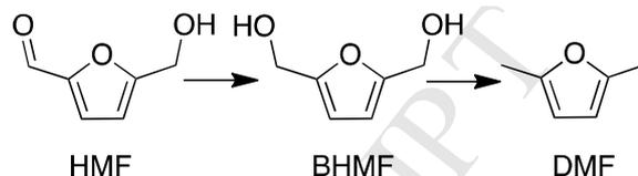
Figure 3. Reduction of HMF to BHMF or DMF.
