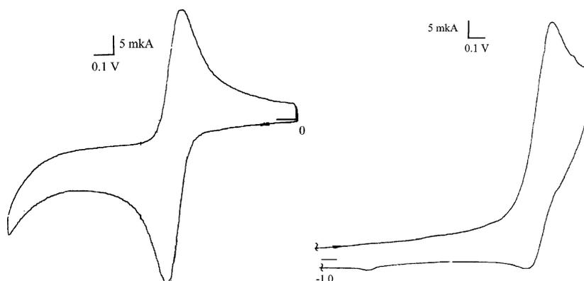
Fig. 1. Cyclic voltammograms of ferrocenylbutyl imidazole (**6**) ( $c=2\times 10^{-3}$  M, with [(*n*-Bu)<sub>4</sub>N]BF<sub>4</sub> in acetonitrile and glassy carbon electrode; the scan rate was 200 mV s<sup>-1</sup>).
