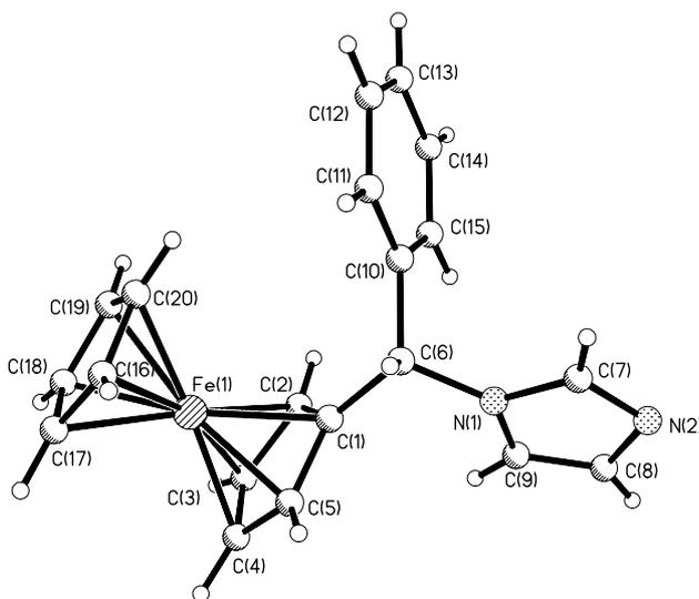
Fig. 3. Molecular structure of ferrocenylbenzyl imidazole (**7**). Selected bond lengths (Å) and bond angles (°): C(1)–C(6)=1.499(5), C(6)–N(1)=1.487(4), C(6)–C(10)=1.521(5), N(1)–C(7)=1.356(5), N(1)–C(9)=1.360(5); C(1)–C(6)–N(1)=108.5(3), C(1)–C(6)–C(10)=115.8(3), N(1)–C(6)–C(10)=109.6(3), C(7)–N(1)–C(9)=105.7(3), C(6)–N(1)–C(7)=124.8(3), C(6)–N(1)–C(9)=129.1(3).
