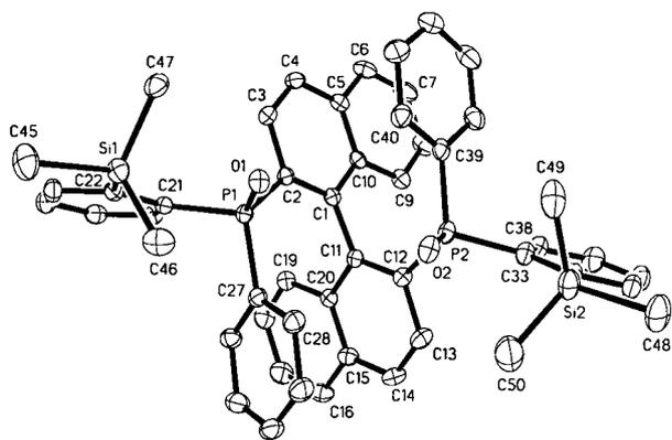
Fig. 5. Solid state structure of **8** (40% ellipsoids, H atoms omitted).
