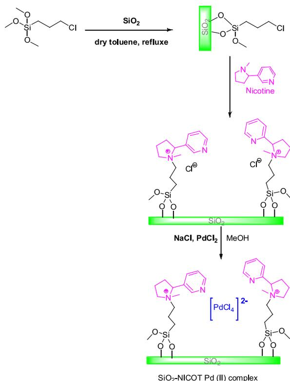
**Scheme 1.** The nanocatalyst preparation.
