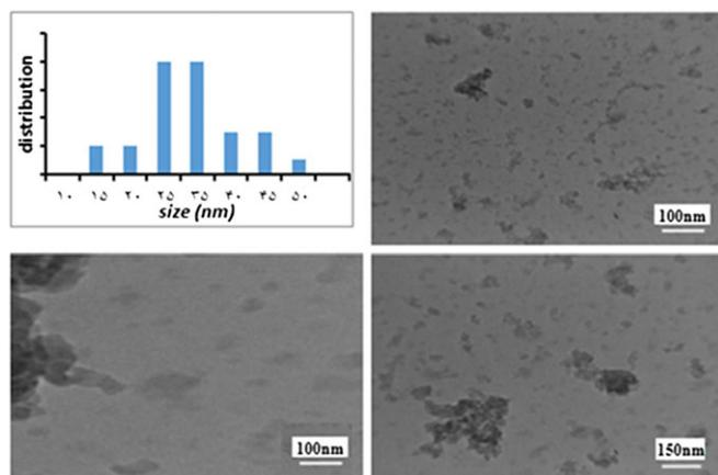
**Figure 3.** TEM images and particle size distribution results for SiO<sub>2</sub>-NICOT-Pd(II) catalyst.
