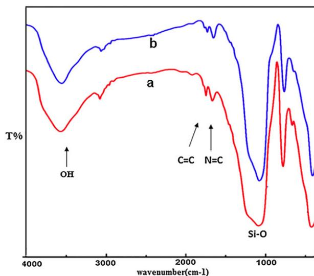
**Figure 1.** FT-IR spectrum of: SiO<sub>2</sub>-NICOT (a) and SiO<sub>2</sub>-NICOT-Pd (b).
