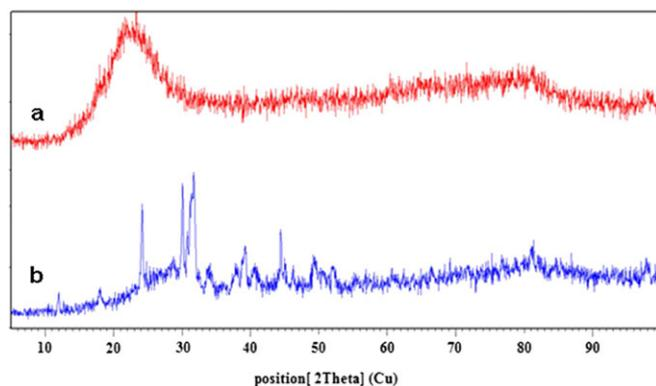
**Figure 4.** XRD pattern of the fresh catalyst (a) and recovered catalyst (b).
