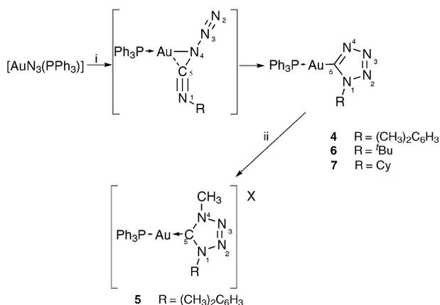
**Scheme 2** The synthesis of C-tetrazolyl gold(I) complexes; X = CF<sub>3</sub>SO<sub>3</sub><sup>-</sup>: (i) RNC = 2,6-Me<sub>2</sub>C<sub>6</sub>H<sub>3</sub>NC, <sup>t</sup>BuNC or CyNC; (ii) CF<sub>3</sub>SO<sub>3</sub>CH<sub>3</sub>.
