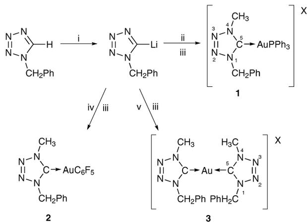
**Scheme 1** The synthetic route towards mono- and bis(tetrazolylidene) gold(I) complexes; X = CF<sub>3</sub>SO<sub>3</sub><sup>−</sup>: (i) *n*-butyllithium in thf; (ii) [AuCl(PPh<sub>3</sub>)]; (iii) CF<sub>3</sub>SO<sub>3</sub>CH<sub>3</sub>; (iv) [Au(C<sub>6</sub>F<sub>5</sub>)(tht)]; (v) [AuCl(tht)].
