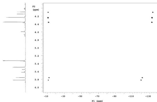
**Fig. 1**  $^1\text{H}$ ,  $^{15}\text{N}$  gHMQC experiment of **1**, collected over a 24 h period in  $\text{CD}_2\text{Cl}_2$  at ambient temperature; for **1** [ $\delta$   $-119.9$  ( $\text{N}^1$ ),  $\delta$   $-11.2$  ( $\text{N}^2$ ),  $\delta$   $-11.5$  ( $\text{N}^3$ ),  $\delta$   $-132.5$  ( $\text{N}^4$ )] and **3** [ $\delta$   $-121.3$  ( $\text{N}^1$ ),  $\delta$   $-12.0$  ( $\text{N}^2$ ),  $\delta$   $-10.9$  ( $\text{N}^3$ ),  $\delta$   $-132.8$  ( $\text{N}^4$ )].
