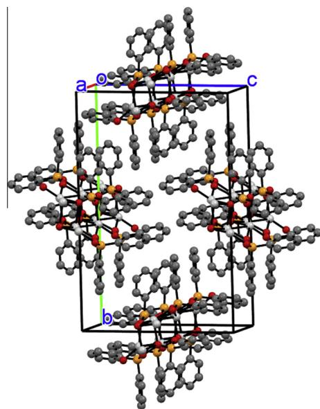
**Fig. 7.** Packing diagram of complex **2** seen along the *bc* plane.
