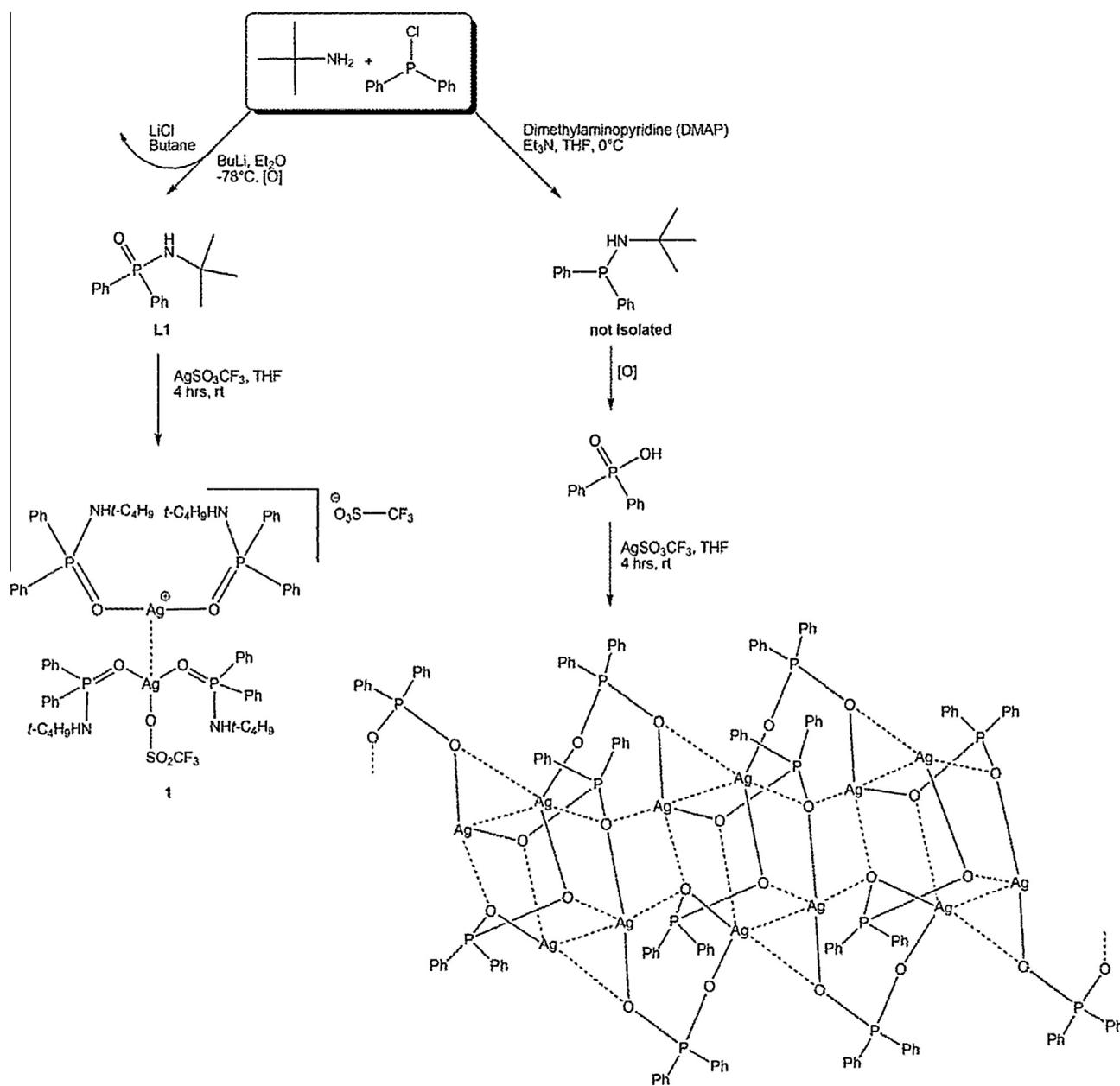
**Scheme 1.** Formation of *N*-*tert*-butyl-diphenylphosphinic amide ligand (**L1**),  $[\text{Ag}(\text{CF}_3\text{SO}_3)(\text{OPPh}_2\text{N}(\text{H})\text{CMe}_3)_2]\{\text{Ag}(\text{OPPh}_2\text{N}(\text{H})\text{CMe}_3)_2\}[\text{SO}_3\text{CF}_3]$  (**1**), and  $[\text{Ag}_2\{((\mu-\text{O})\text{OPPh}_2)_2\text{O}_2\text{PPh}_2\}][\text{SO}_3\text{CF}_3]$ , (**2**).
