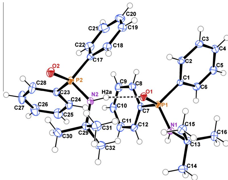
**Fig. 1.** Ligand **L1** shown as dimer with atom labeling. The displacement ellipsoids are shown at the 50% probability level.
