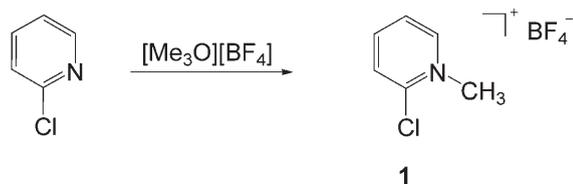
**Scheme 1.** Alkylation of chloropyridines according to Stone.<sup>[12]</sup>
