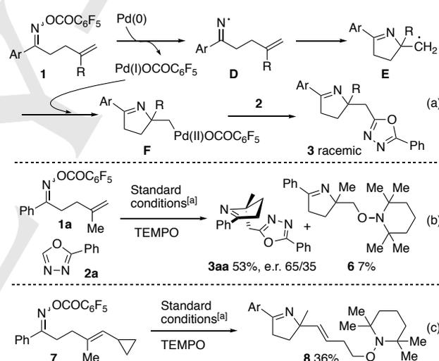
**Scheme 6.** Possible competitive radical mechanism and results of control experiments. [a] **1a** (0.2 mmol), **2a** (0.1 mmol), TEMPO (0.2 mmol), Pd(OAc)<sub>2</sub> (0.1 equiv), (S)-Synphos (0.2 equiv), K<sub>2</sub>CO<sub>3</sub> (0.3 mmol), DMSO (1.0 mL), 100 °C, 8 h.
