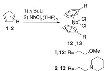
**Scheme 1.** Synthesis of niobocene dichlorides **12** and **13**.
