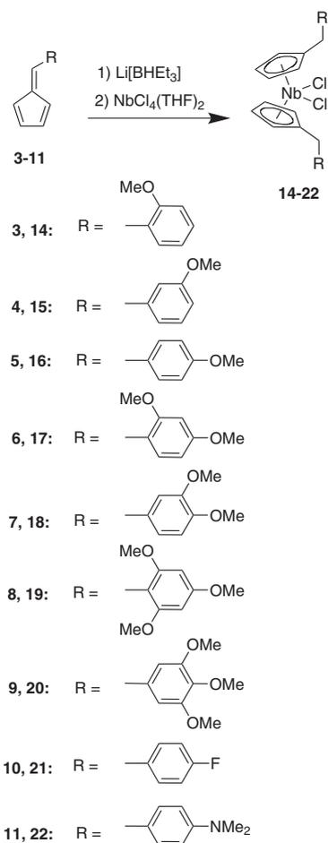
**Scheme 2.** Synthesis of niobocene dichlorides **14**–**22**.
