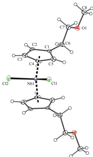
**Figure 2.** Molecular structure of (MeOCH<sub>2</sub>CH<sub>2</sub>C<sub>5</sub>H<sub>4</sub>)<sub>2</sub>NbCl<sub>2</sub> (**12**) showing the labeling scheme for all non-hydrogen atoms. Anisotropic displacement ellipsoids are drawn at the 30% probability level. Unlabeled atoms are related by symmetry operation:  $-x; -y, \frac{1}{2} + z$ .
