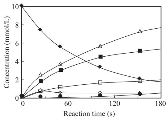
**Figure 3** Effect of reaction time on the concentration of products obtained by hydrothermal decomposition of aspartic acid at 220°C (◆: aspartic acid, △: ammonia, ■: fumaric acid, □: maleic acid, ◇: pyruvic acid, and ●: malic acid).
