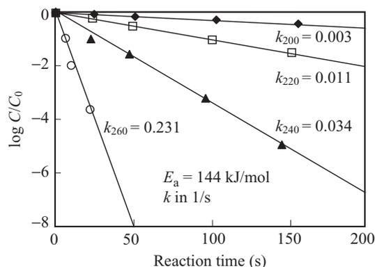
**Figure 2** First-order kinetic plots of hydrothermal decomposition of aspartic acid (◆: 200°C, □: 200°C, ▲: 240°C, and ○: 260°C).
