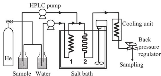
**Figure 1** Schematic diagram of continuous-flow tubular reactor apparatus for experiments with high-temperature and high-pressure water (1: preheater and 2: reactor).
