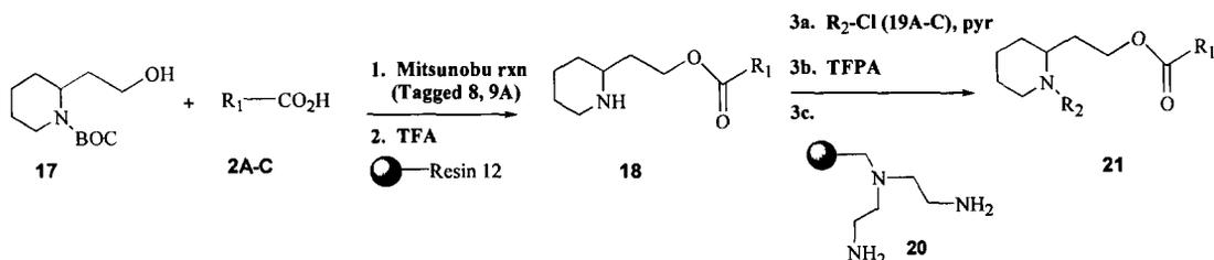
As Table 2 illustrates, good mass yields (47–60%) were obtained using the tagged Mitsunobu reagents in this three step array synthesis. Purities, as determined by proton NMR and HPLC, were exceptional (95–100%). In particular, proton NMR showed no sign of contamination of the final products **21** with any of the tagged reagents or reagent byproducts. Moreover, the concomitant use of TFPA allowed products to be obtained free from starting alcohol impurities.
