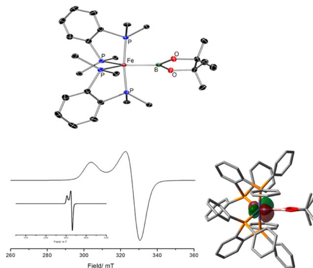
**Figure 1.** (top) X-ray structure of **2**, with H atoms and C atoms except for the ipso-C atoms of Ph residues omitted. Ellipsoids were set at 50% probability. (bottom left) X-band EPR spectrum (THF, 140 K) of **2**. (bottom right) Calculated SOMO (isovalue  $\pm 0.05$  (electron/ $\text{bohr}^3$ )<sup>1/2</sup>) of low-spin **2**.<sup>9</sup>
