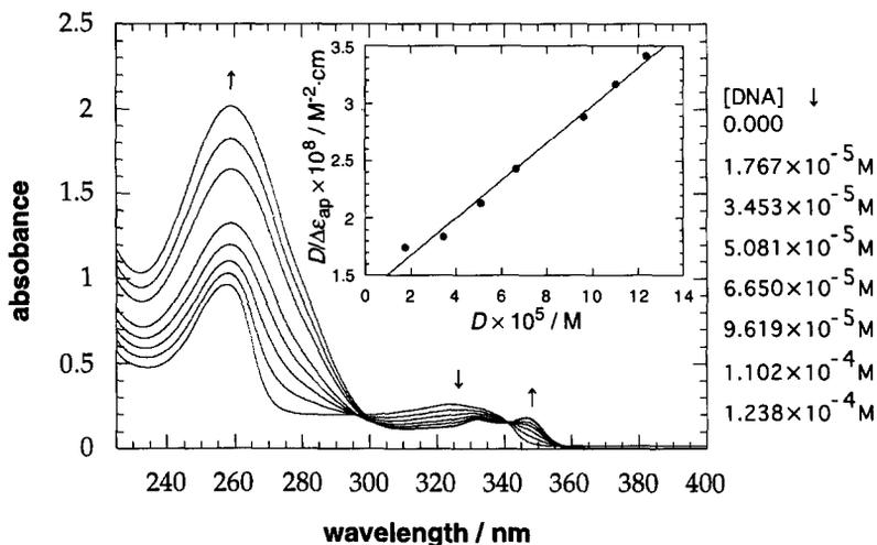
**Figure 1.** Absorbance change of compound **4** ( $2.5 \times 10^{-5} M$ ) in the presence of increasing amount of calf thymus DNA in 1.0 mM sodium cacodylate buffer containing 4.0 mM NaCl (pH 6.0) at 25 °C. Inset: Plot of  $D/\Delta\epsilon_{ap}$  vs  $D$  at 325 nm. See text.
