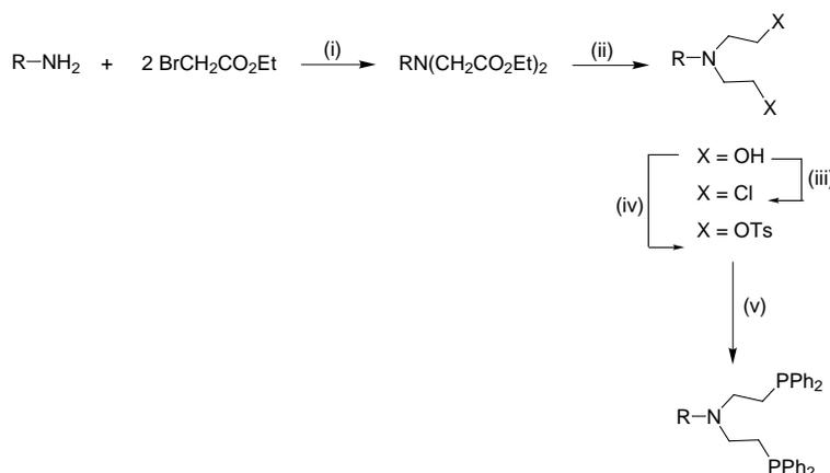
Preparation of aminodiphosphine ligands; Reagents and conditions: (i) Na<sub>2</sub>CO<sub>3</sub>, EtOH, reflux; (ii) LiAlH<sub>4</sub>; (iii) SOCl<sub>2</sub>; (iv) TsCl, pyridine; (v) KPPH<sub>2</sub>
