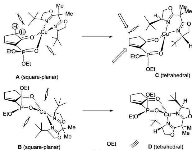
**Figure 3.** Proposed models for the catalytic asymmetric Michael reaction of the L4–Cu(II)–1c complex.
