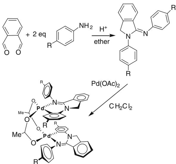
**Scheme 1.** Synthesis of iminoisoindoline ligands and corresponding acetato-bridged dinuclear palladacycles.
