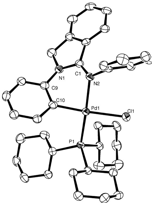
**Fig. 3.** ORTEP plot of **12** at the 50% probability level. The hydrogen atoms have been omitted for clarity. Selected bond lengths [Å] and angles [°]: Pd(1)–C(10) = 1.995(3), Pd(1)–N(2) = 2.130(3), Pd(1)–Cl(1) = 2.4077(9), Pd(1)–P(1) = 2.2901(8), C(10)–Pd(1)–N(2) = 84.26(12), C(10)–Pd(1)–Cl(1) = 174.30(9), N(2)–Pd(1)–Cl(1) = 91.17(8), C(10)–Pd(1)–P(1) = 94.38(9), N(2)–Pd(1)–P(1) = 166.64(8), Cl(1)–Pd(1)–P(1) = 90.85(3).
