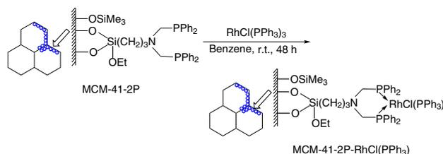
**Scheme 1.** Preparation of MCM-41-2P-RhCl(PPh<sub>3</sub>) complex.
