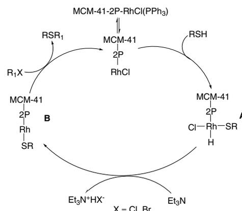
**Scheme 3.** Plausible mechanism of reaction catalyzed by heterogeneous rhodium.
