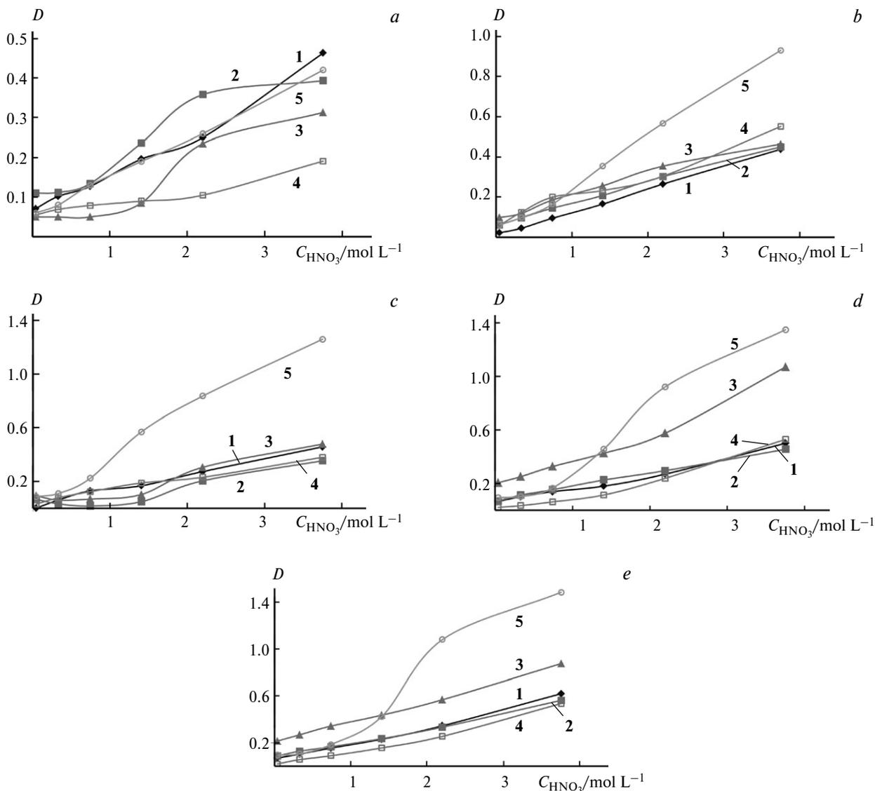
**Fig. 1.** Dependence of distribution ratios for  $U^{VI}$  (a),  $La^{III}$  (b),  $Nd^{III}$  (c),  $Ho^{III}$  (d), and  $Yb^{III}$  (e) from the concentration of  $HNO_3$  in the extraction with phosphorylureas 1–5 (0.01 M solution in  $CHCl_3$ ).
