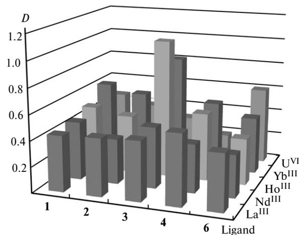
**Fig. 2.** Comparison of distribution ratios of  $\text{La}^{\text{III}}$ ,  $\text{Nd}^{\text{III}}$ ,  $\text{Ho}^{\text{III}}$ ,  $\text{Yb}^{\text{III}}$ , and  $\text{U}^{\text{VI}}$  in the extraction with ligands **1–4** and **6** ( $0.01\text{ M}$  solutions in  $\text{CHCl}_3$ ) from  $3.75\text{ M}$   $\text{HNO}_3$ , the initial concentration of lanthanide and uranyl nitrates in aqueous phase was  $2.5 \cdot 10^{-4}\text{ mol L}^{-1}$ .
