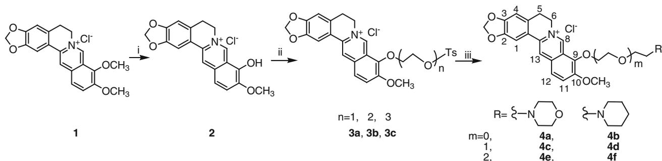
**Scheme 1** Synthesis of berberine derivatives. (i) 190  $^{\circ}\text{C}$ , 20–30 mmHg, 20 min; (ii)  $\text{CH}_3\text{CN}$ ,  $\text{K}_2\text{CO}_3$ ,  $\text{TsO}(\text{CH}_2\text{CH}_2\text{O})_n\text{Ts}$  ( $n = 1, 2, 3$ ), 60  $^{\circ}\text{C}$ , 3 h; (iii) morpholine (or piperidine),  $\text{CH}_3\text{CN}$ ,  $\text{K}_2\text{CO}_3$ , 80  $^{\circ}\text{C}$ , 2–3 h
