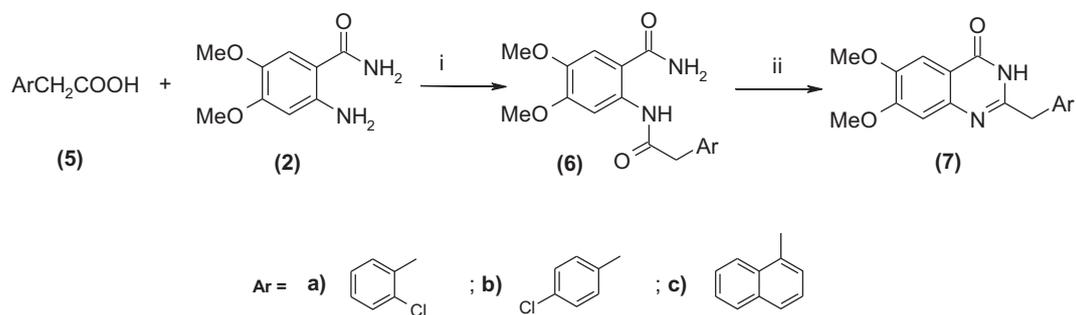
**Scheme 2.** Reagents and conditions: i)  $\text{SOCl}_2$ , 1,4 Dioxane; ii)  $t\text{-BuONa}$ , ethylene glycol, MW.
