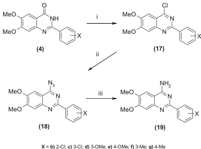
**Scheme 5.** Reagents and conditions: i) POCl<sub>3</sub>, DMF; ii) NaN<sub>3</sub>, DMF, mw; iii) H<sub>2</sub>/Pd/C, CH<sub>3</sub>OH.
