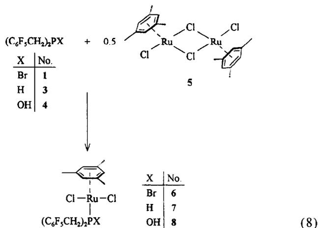
In contrast to the starting phosphorus(III) compounds **1**, **3** and **4**, the complexes formed were neither air- nor moisture-sensitive. The identity of compounds **6–8** was established by infrared and NMR spectroscopy ( $^1\text{H}$ ,  $^{13}\text{C}$ ,  $^{19}\text{F}$ ,  $^{31}\text{P}$ ), mass spectrometry and elemental analysis, and, in the case of **8**, by a single-crystal X-ray structure determination.
