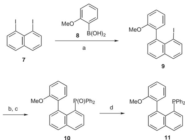
**Scheme 2** Preparation of phenylnaphthyl phosphine **11**. *Reagents and conditions:* a) Pd(PPh<sub>3</sub>)<sub>4</sub> (5.0 mol%), Cs<sub>2</sub>CO<sub>3</sub>, toluene–EtOH–H<sub>2</sub>O (3:2:2), 100 °C, 66%; b) *n*-BuLi, Et<sub>2</sub>O, –78 °C; c) Ph<sub>2</sub>P(O)Cl, Et<sub>2</sub>O, –78 to 50 °C, 62% (two steps); d) HSiCl<sub>3</sub>, Et<sub>3</sub>N, xylene, 120 °C, 34%.
