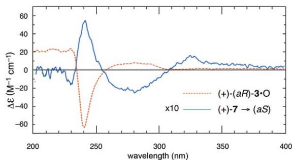
**Figure 3** Comparison of electronic CD spectra for phosphine oxides (+)-**7** and (+)-(*aR*)-MOP-oxide (**3-O**) collected from MeOH solutions (0.30 mM and 0.17 mM, respectively). Phosphine oxide (+)-**7** was assigned as having (*aS*)-configuration because this material shows an opposite exciton chirality phase to that exhibited by (+)-(*aR*)-MOP-oxide.
