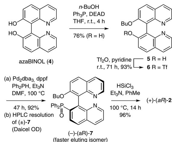
**Scheme 1** Synthesis of (+)-(aR)-2 from 7,7'-dihydroxy-8,8'-biquinolyl ('azaBINOL', 4)
