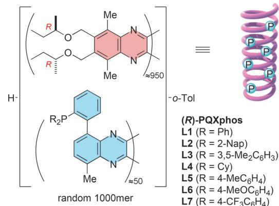
Figure 1. The poly(quinoline-2,3-diyl)-based helically chiral phosphine ligand *PQXphos*.
