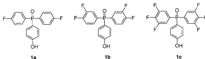
**Figure 1.** AB<sub>2</sub> monomers, **1a**, **1b**, and **1c**, utilized to prepare hyperbranched poly(arylene ether phosphine oxide)s via nucleophilic aromatic substitution reactions.
