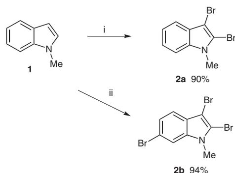
**Scheme 1** Bromination of *N*-methylindole (**1**). Reagents and conditions: i, NBS (2.1 equiv), THF, –78 °C, 4 h; ii, NBS (3.1 equiv), THF, –78 °C, 4 h, then 20 °C, 14 h.
