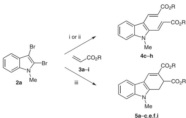
**Scheme 2** Synthesis of **4c–h** and **5a–c,e,f,i**. Reagents and conditions: *i*, for **4c–g**: Pd(OAc)<sub>2</sub> (5 mol%), L (10 mol%), Et<sub>3</sub>N, DMF, 90 °C, 36 h; *ii*, for **4h**: Pd(OAc)<sub>2</sub> (5 mol%), N(CH<sub>2</sub>CH<sub>2</sub>OH)<sub>3</sub> (3 mL), 90 °C, 36 h; *iii*, Pd(OAc)<sub>2</sub> (5 mol%), L (10 mol%), Et<sub>3</sub>N (8.0 equiv), DMF, 120 °C, 48 h.
