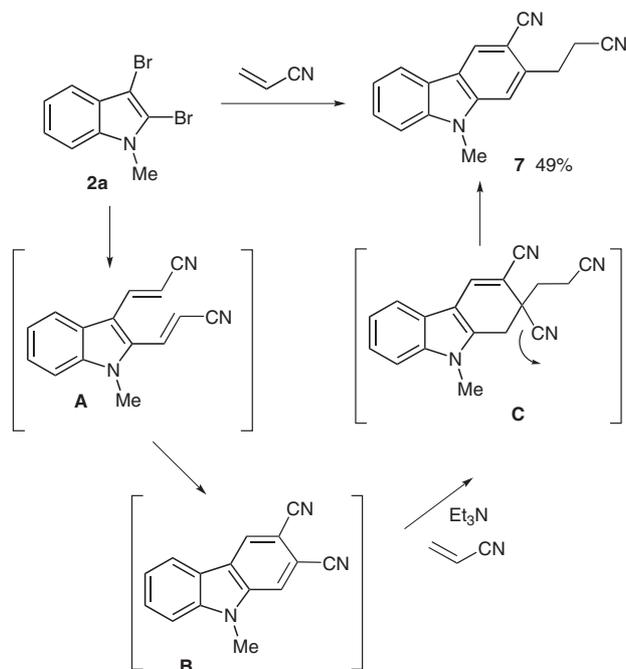
**Scheme 4** Possible mechanism of the formation of **7**. *Reagents and conditions:* i, Pd(OAc)<sub>2</sub> (5 mol%), **L** (10 mol%), Et<sub>3</sub>N, DMF, 120 °C, 48 h.
