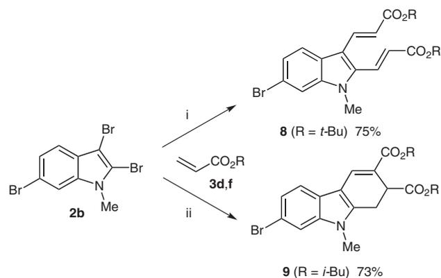
**Scheme 5** Synthesis of **8** and **9**. *Reagents and conditions:* i, Pd(OAc)<sub>2</sub> (5 mol%), **L** (10 mol%), Et<sub>3</sub>N, DMF, 90 °C, 24 h; ii, Pd(OAc)<sub>2</sub> (5 mol%), **L** (10 mol%), Et<sub>3</sub>N, DMF, 120 °C, 48 h.
