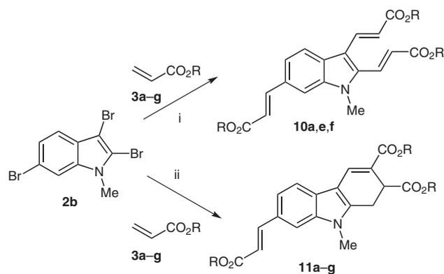
**Scheme 6** Synthesis of **10a,e,f** and **11a–g**. *Reagents and conditions:* i, Pd(OAc)<sub>2</sub> (5 mol%), **L** (10 mol%), Et<sub>3</sub>N, DMF, 90 °C, 36 h; ii, Pd(OAc)<sub>2</sub> (5 mol%), **L** (10 mol%), Et<sub>3</sub>N, DMF, 120 °C, 48 h.
