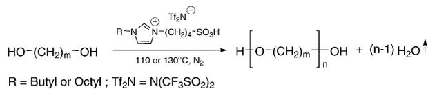
**Scheme 1** Synthesis of linear polyether in 4-(3'-butyl-1'-imidazolio)-1-butanedisulfonic acid bis(trifluoromethylsulfonyl)imidide ([RBSIm][Tf<sub>2</sub>N], *m* > 6).
